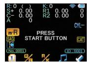
**Axis Correction Function** An internal sensor detects the inclination of the instrument to display the automatically corrected axis.\*
