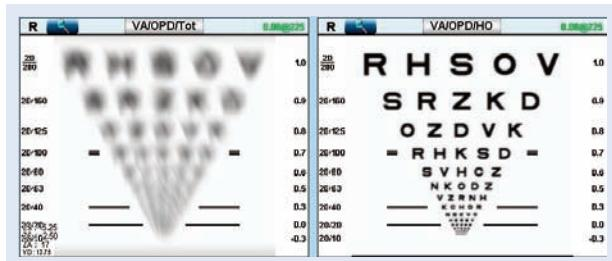
Figure 3. The visual acuity display on the OPD-Scan III provides comparative images with and without higher-and/or lower-order aberration corrections.
